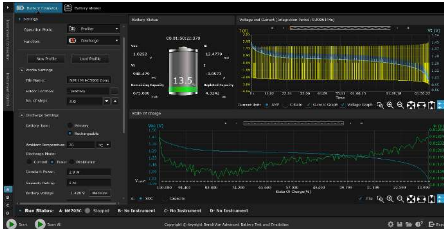
Figure 4. Creating a battery profiler with ambient temperature and constant power discharge features.
